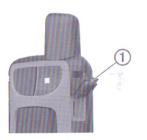
2 Insert the memory card with the gold contacts facing the front of the device.
